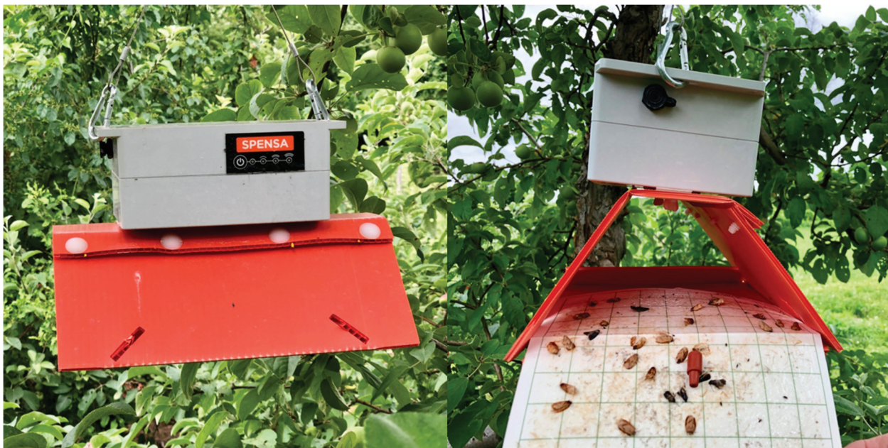
Figure 1. Smart Traps in an apple orchard block at the UMass Orchard with oblique banded leafroller pheromone catch.
