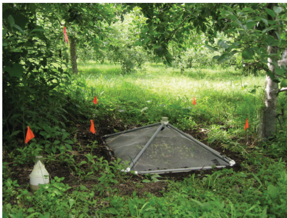
Figure 1. Depiction of the PVC enclosure (left) and pyramidal emergence cage (1 × 1 yards at the base) (center) used for the evaluation of entomopathogenic nematodes (EPNs) in the second study.
