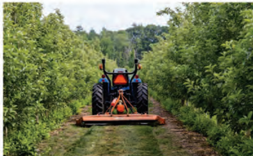
RAS-Rotary Mower. Ideal for mowing orchard rows.
