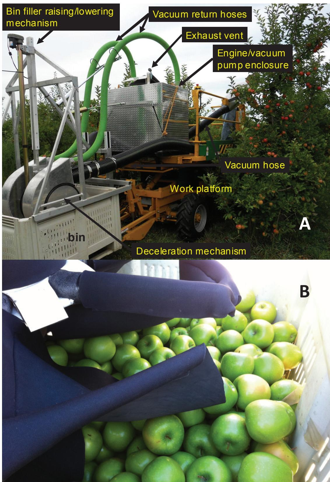
Figure 1. A. Components of vacuum-assisted harvest system. B. Elephant-ear distributor in motion.
