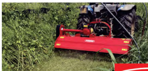
Shredder/Flail Mowers Ideal for chipping brush, managing field edges, handling cover crops
