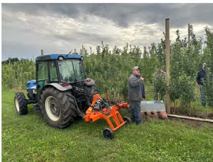
Photo 1. Trevor Hardy demonstrates The Rinieri Biodynamic SRL mechanical weeder which makes short-work of weeds and apple rootsuckers at Brookdale Fruit Farm. Sold by Brookdale Farm Supply . Photo Credit: Win Cowgill.
